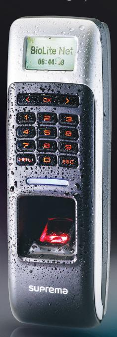
BioLite Net Suprema introduces BioLite Net, the world's smallest IP-based fingerprint terminal with time attendance and access control capability. With rugged IP65 rated waterproof structure, it offers extra durability and it's perfect for outdoor installation. From simple door control to complex networked environment, BioLite Net supports full functionality of time attendance and access control. All features comes in an elegantly designed, slick and slim device.
